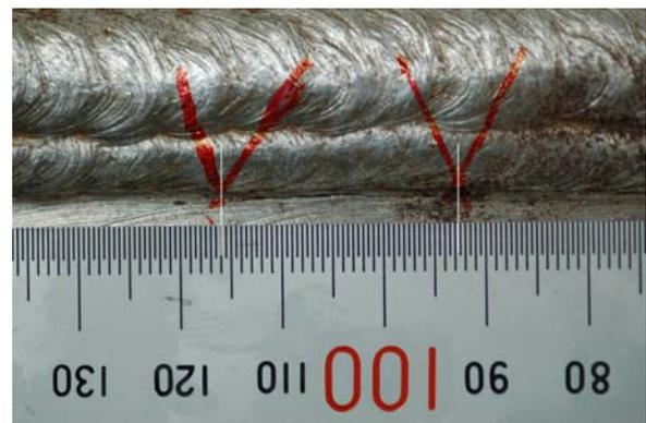
Figure 15: *Result of crack sizing*
