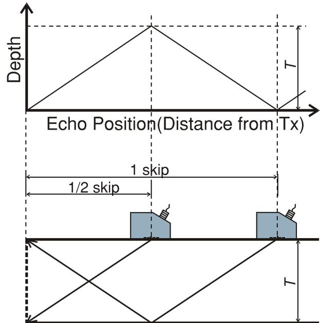
Figure 3: *Depth according to echo position.*
