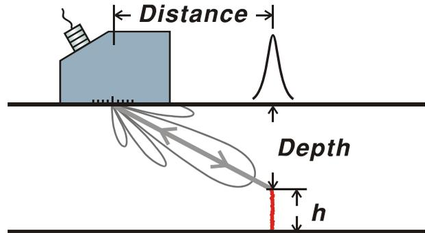
Figure 6: Measurement of crack height.
