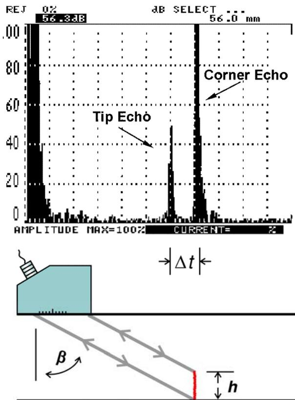
Figure 5: Satellite pulse technique.
