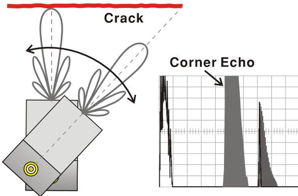
Figure 8: Swivel scan at in of crack.
