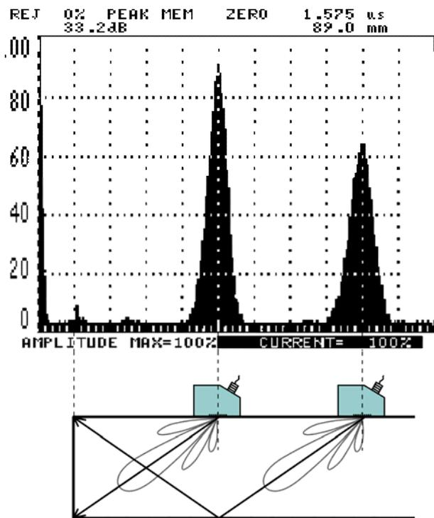
Figure 2: *Beam profile effect at corners.*
