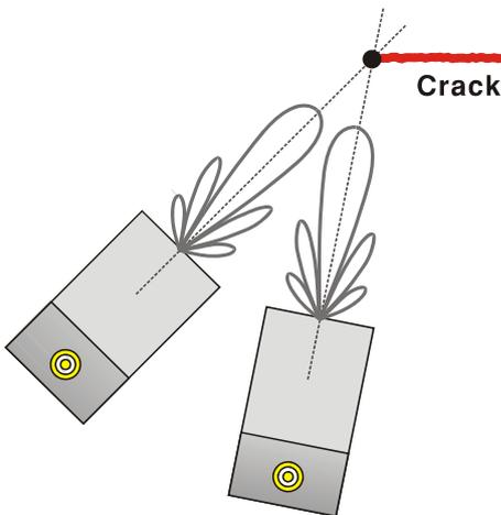
Figure 9: End of crack detected by line crossing.
