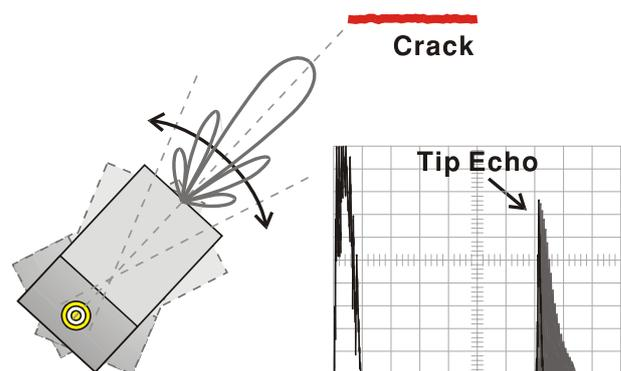
Figure 7: Swivel scan at out of crack.
